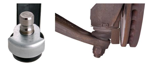
Heat shields occur on cars with ball joints with cylindrical pins on brands like Citroën, Dacia, Ford, Mazda, Nissan, Peugeot, Renault,...
