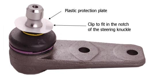
Protection plates occur on cars with ball joints with cylindrical pins mainly on Renault applications.
