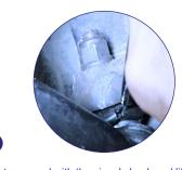
Next, proceed with the visual check and lift the car First, check the condition of the dust cover on the ball joint.
