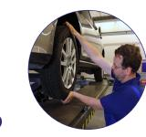
At the start of the visual check, lift the car until the wheels come off the ground.
