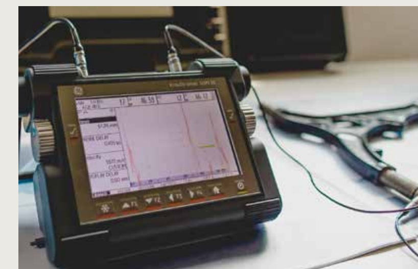
Ultrasonic crack control for casting parts
